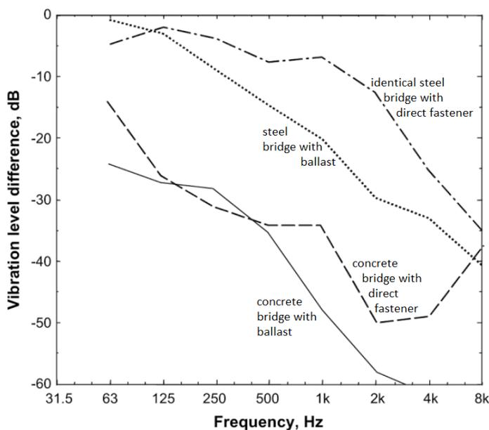
Figure 8 Measured vibration level difference between rail and bridge. Figure copied from [2], used by kind permission of David Thompson.
