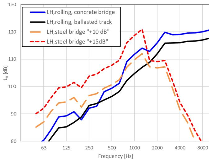
Figure 7 Rolling noise and bridge noise transfer functions.
