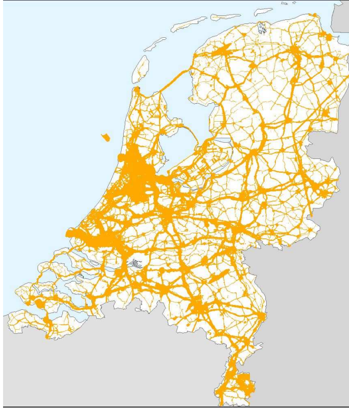
Figure 2 – Dutch noise footprint (50 dB L_{den} contour). This map includes wind turbine noise at sea. After [2].
