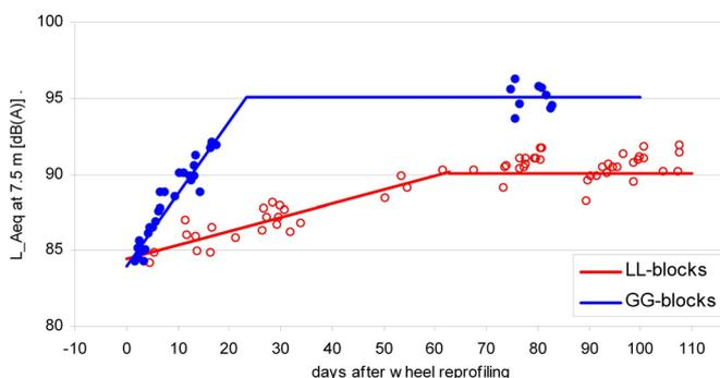
**Figure 2:** Increase of rolling noise due to growth of wheel roughness after reprofiling. Results for passenger trains (ICR type) with cast-iron blocks (GG) and LL-blocks. Each colour represents a fixed set of ICR vehicles followed in time at one site.
