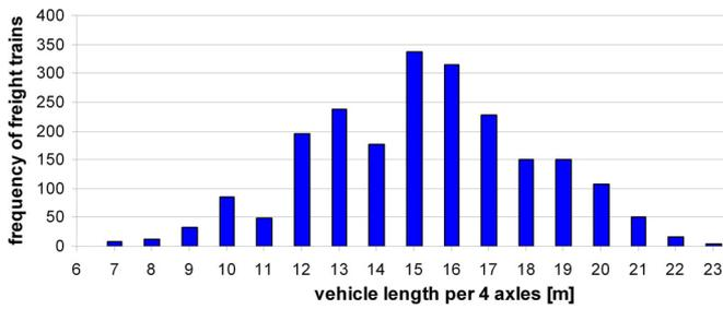
**Figure 1:** Distribution of average vehicle length of freight trains in the Netherlands. Lengths refer to 4 axles, so not necessarily from buffer to buffer.
