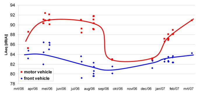
**Figure 3:** Long-term variations for the two outer vehicles of an EMU of type mDDM with serious wheel defects at the motor unit. After a maintenance action around September 2006 the problem occurred again in February 2007. The measurements were taken at different sites and where not corrected for rail roughness differences.
