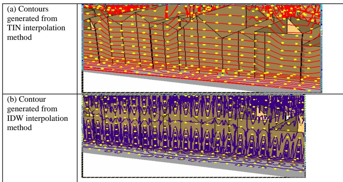
Figure 6: Noise contours of two interpolation methods projected on 3D city model
