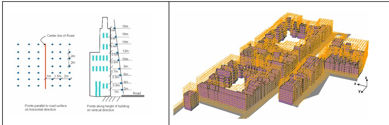
**Figure 3: (a) spacing of points in horizontal and vertical direction on facades of building, (b) observation points to be used as basis for interpolated noise surface**
