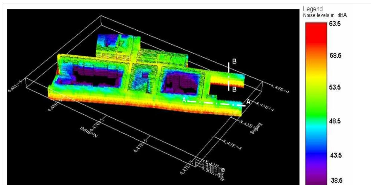
Figure 9: Volumetric view of noise levels on the road surface of study area
