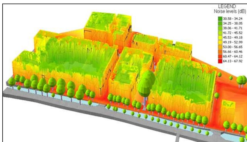
Figure 5: 3D noise map obtained with TIN interpolation
